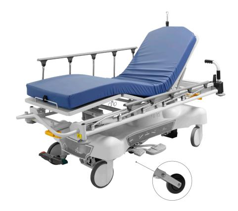
The Amico Hydraulic Patient Transfer Stretcher (S-H-300) provides caregivers the control they need in the emergency environment. The stretchers can be adjusted to various positions – raising, lowering, trendelenburg, and reverse trendelenburg – by actuating the hydraulic pistons. The back section is adjustable through the use of gas springs and the knee gatch can be raised and lowered with an optional manual crank.
